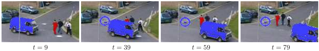
Fig. 9. Truck and pedestrian sequence \mu = 1 , \beta_i = \beta = 1.5 and \gamma = 2.0 : The pedestrian is well tracked, but the bad segmentations are not rejected, as no error is taken into account on the local motion of the interest points.
