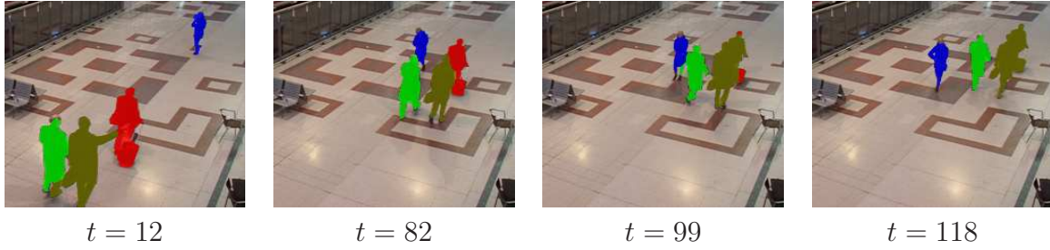
Fig. 15. People in the station sequence - results with standard parameters: \mu = 1.5 , \beta = 2.5 and \gamma = 0.5 . The algorithm fails by merging two pedestrians.
