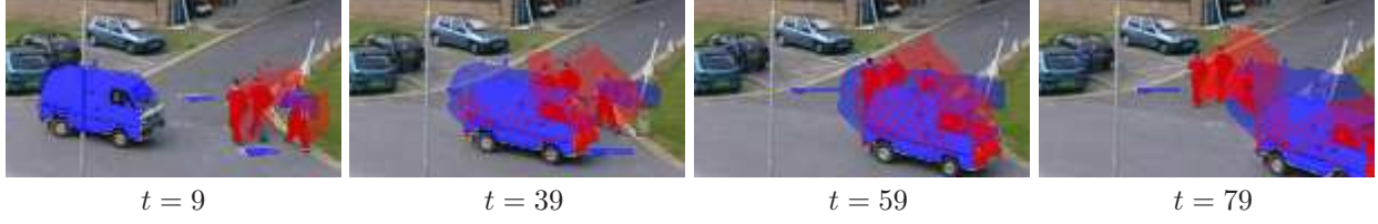
Fig. 10. Truck and pedestrian sequence with standard parameters \mu = 1.5 , \beta = 2.5 and \gamma = 0.5 : The small value of the parameter \gamma leads the process to search for the target too far away from the predictions.
