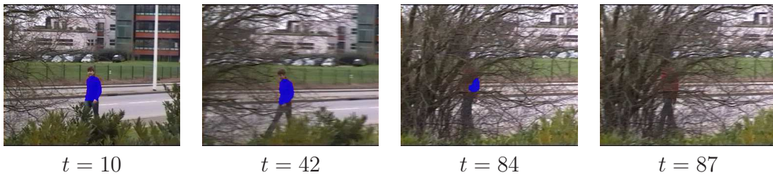
Fig. 19. Man behind tree sequence - results with [23]: R_p = 0 , \mu = 0 , \beta_i = 0 and \gamma = 0.5 . The target is lost after the first total occlusion.
