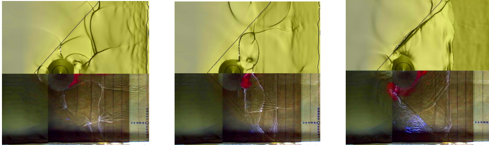
Figure 26: Solitary wave on a shelf (RD scheme). Comparison between numerical solution and experiment.
