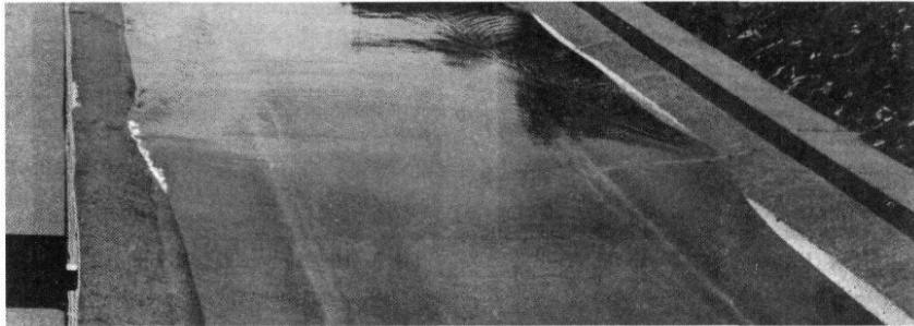
Fig. 8. Undular bore at Froude ~ 1.04.
