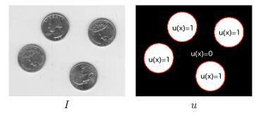
The segmentation of the image I is represented by the binary mask u. The foreground region  $S_u = \{x, u(x) = 1\}$  (in white in the right image), corresponds to the coins which mean color in I is  $c_1 = 110$ . The background region is represented by  $\{x, u(x) = 0\}$  (in black in the right image). It is associated to the mean color  $c_2 = 227$  in I. The boundary  $\partial S_u$  between both regions (in red) represents the contour of interest.
