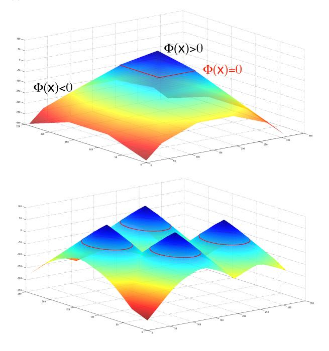
Examples of level set functions  $\phi$  whose zero level set  $\{x, \phi(x) = 0\}$  (in red) represents a contour of interest  $\partial S_u$  in the image domain. The object of interest is represented by the pixels  $\phi(x) > 0$  (in blue). The objects are: a square (top) and the 4 coins of previous example (bottom).
