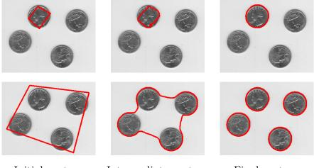
Initial contour Intermediate contour Final contour
