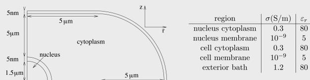
Figure 1: 1/4 of the geometry of the cell considered in this work (z-axis is an axis of revolution) and its electrical parameters.
