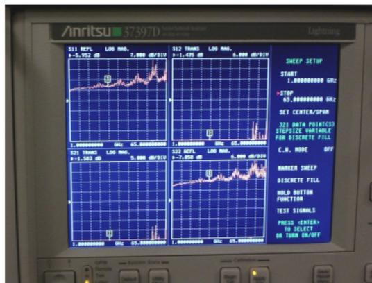
VNA (Vector Network Analyzer) - Magnitude of S-parameters for 2 ports
