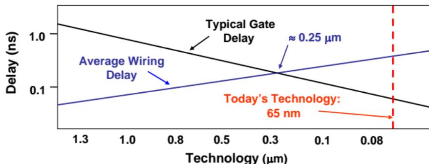
**65nm technology: gate delay < interconnect delay!**
