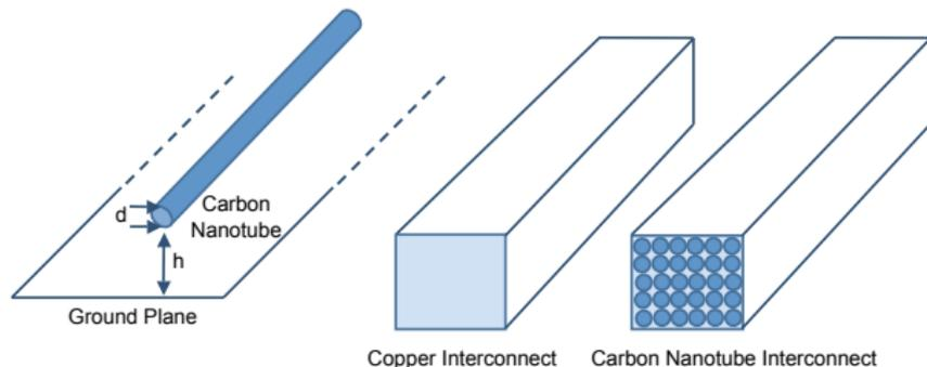
Analytical model of SWCNT: transmission line involving magnetic and kinetic inductance, as well as electrostatic and quantum capacitance.
