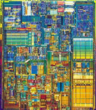
A color micrograph of the Intel Pentium IV microprocessor. The chip is extremely dense and complex, with a wide variety of colors (blue, yellow, green, red) used to highlight different functional blocks and interconnects, illustrating the massive scale of VLSI technology. |
