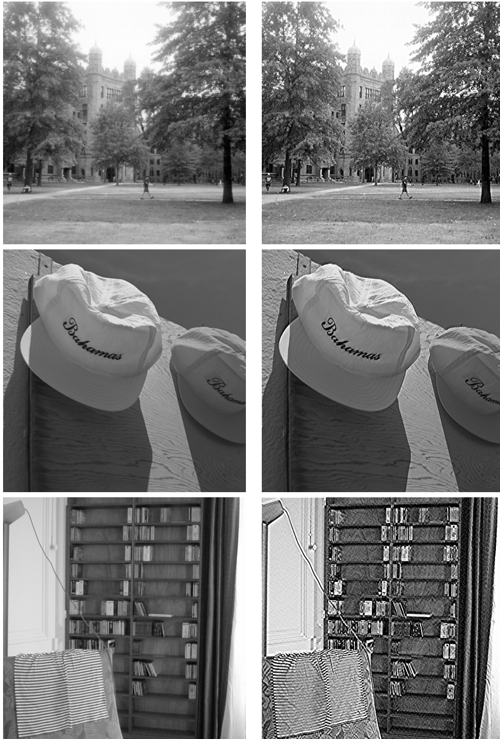
Figure 4.13: Blind deblurring results obtained by running Algorithm 2 on the set of 11 \times 11 kernels. The original (unprocessed) images are shown on the left column (from top to bottom: Yale , Caps (cropped), Room ), and the sharpened images are displayed on the right column. In the first two cases, the output image is sharper than the original one and presents a limited quantity of ringing artifacts. However, the result is not satisfactory for the Room image.
