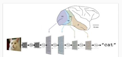
A deep neural network consists of a hierarchy of layers, whereby each layer transforms the input data into more abstract representations (e.g. edge -> nose -> face). The output layer combines those features to make predictions.
