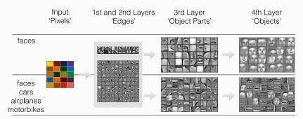
Each layer progressively extracts higher level features of the input until the final layer essentially makes a decision about what the input shows. The more layers the network has, the higher level features it will learn.
