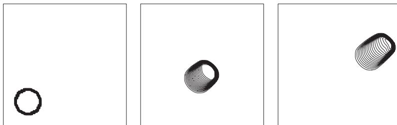
Figure 3. Convection in an oblique velocity field with a quadratic adsorption. Concentration contours of the initial condition (left), numerical solution at times  $t = 0.2$  (centre) and  $t = 0.4$  (right), using twenty isovalues between 0 and 1.
