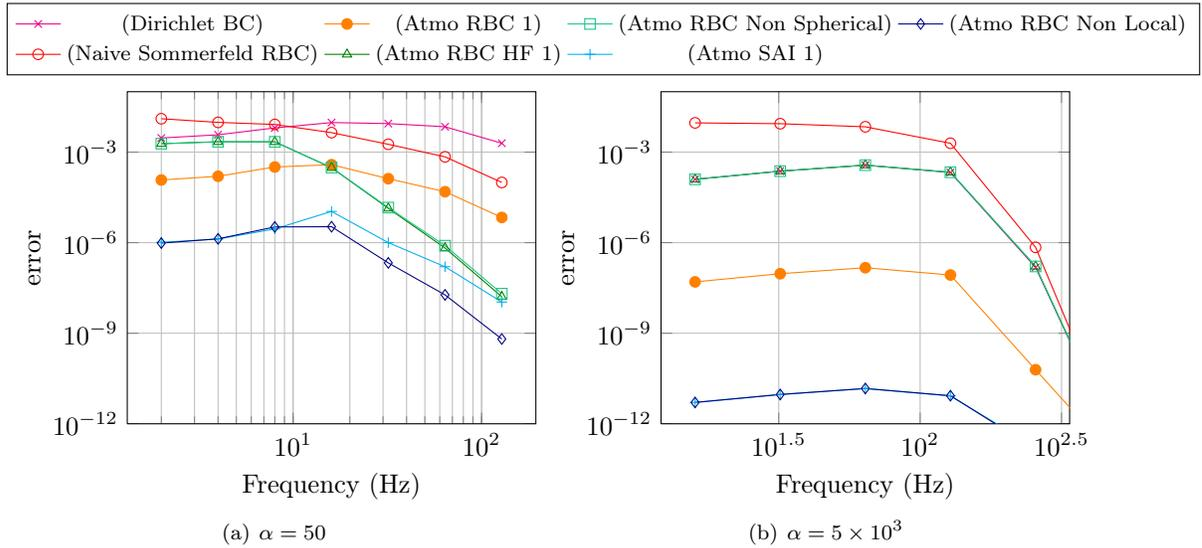
FIGURE 5.  $L^2$  relative errors with reference solution, with respect to the frequency.
