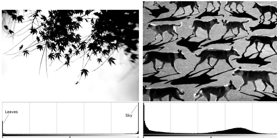
Figure 7.1: Histograms of a low contrast (first column) high contrast (second column) image.
