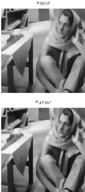
Figure 4. u component of TV - L^2 and TV - G decompositions of the Barbara image (the TV - G decomposition is approximated with the A^2BC algorithm).
