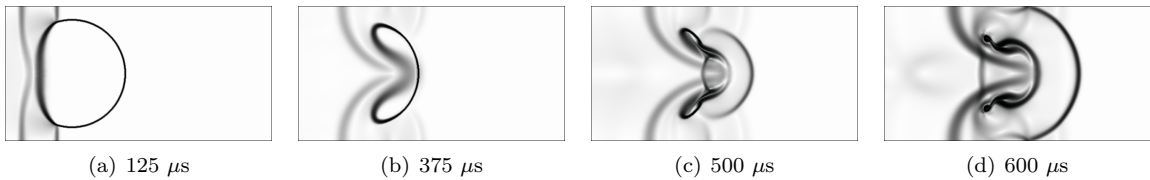
Figure 17: Two-dimensional liquid-gas interaction: Schlieren images, IMEX scheme.
