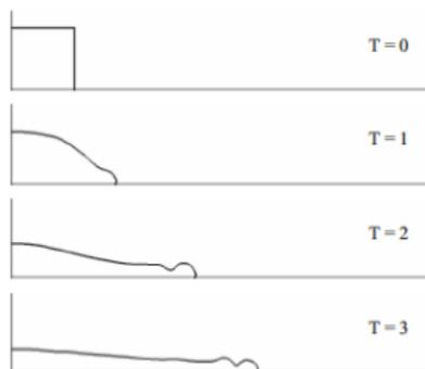
Dam break test case : propagation
