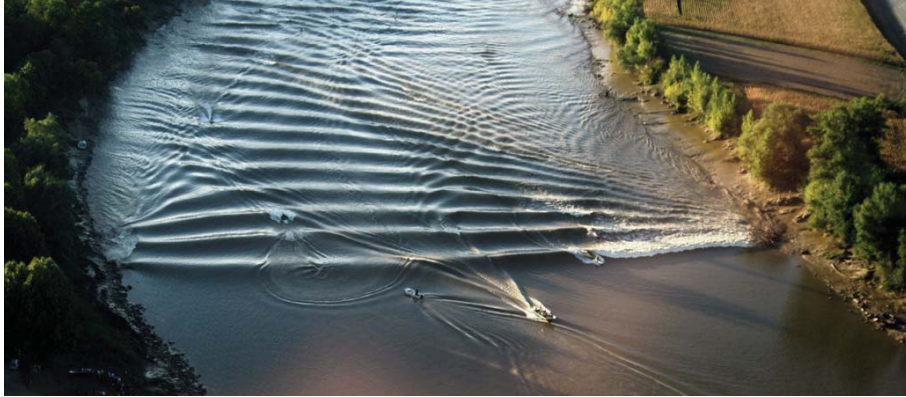
Figure 1: Illustration of a tidal bore propagating in the Garonne River. Aerial photograph taken at Podensac on September 10, 2010. Tidal wave amplitude at the estuary mouth A_0 = 2.5 m and freshwater discharge q_0 = 128 m^3/s
