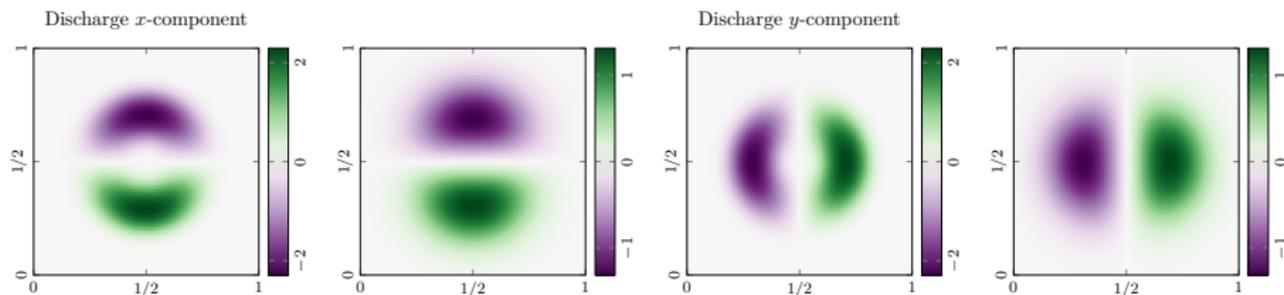
**Figure:** Improved results when replacing  $L^{\text{Rusanov}}$  by second order centered differences  $L^\star$
