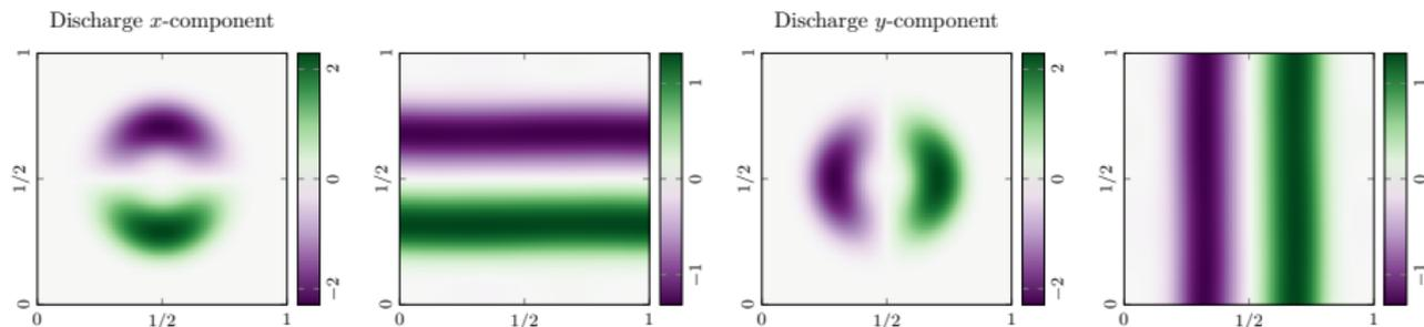
Figure: Steady vortex over non flat bottom,  $100 \times 100$  mesh,  $\text{Fr} = 10^{-2}$ .
