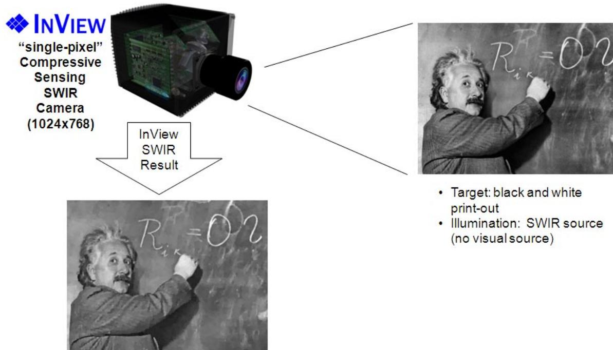
Figure 8: SWIR Reconstruction using  $m = .5N^2$  measurements
