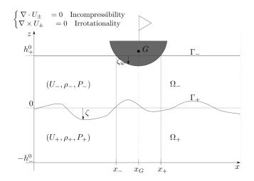
Original Newton's equation :  $m\ddot{x}_G = F_0 + F_P$  with  $F_P = -\int_{\mathbb{R}} P_{z=h_-^0 + \zeta_w} \partial_x \zeta_w dx$ Shallow water regime, we have  $P_{|z=\zeta_w} = \underline{P} + \rho_- gh_-$ , i.e. the non-hydrostatic component is neglected.
