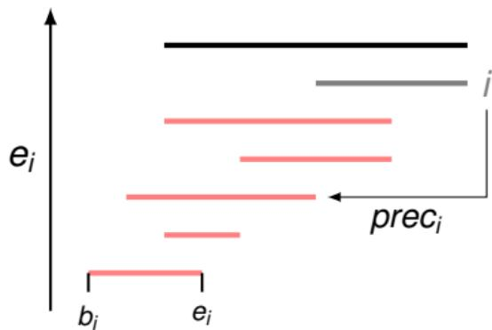
$$P(i, w) = \max \{ P(prec_i, w - w_i) + p_i, P(i - 1, w) \}$$
