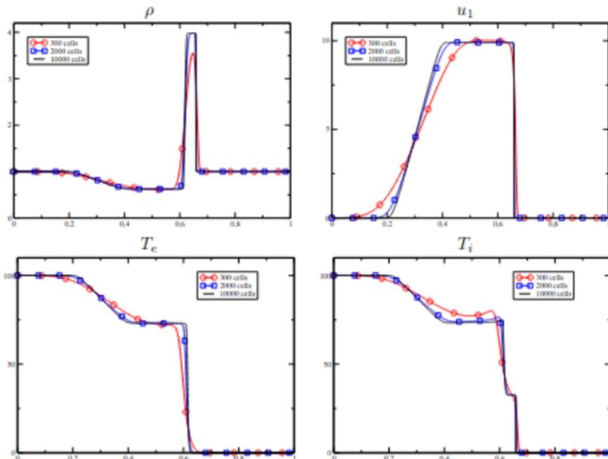
a strong wave of shock, a contact surface and a left rarefaction wave
