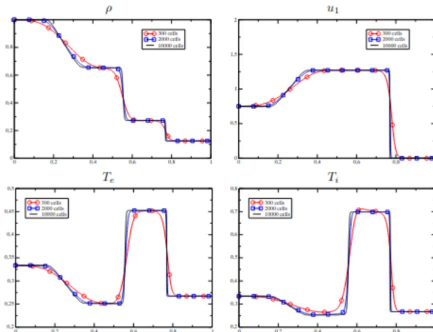
right shock wave, a right travelling contact and a left sonic rarefaction wave
