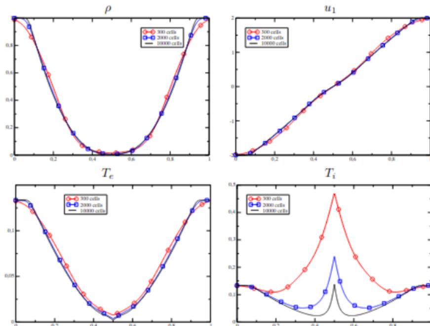
two symmetric rarefaction waves travelling in opposite direction and a trivial contact wave
