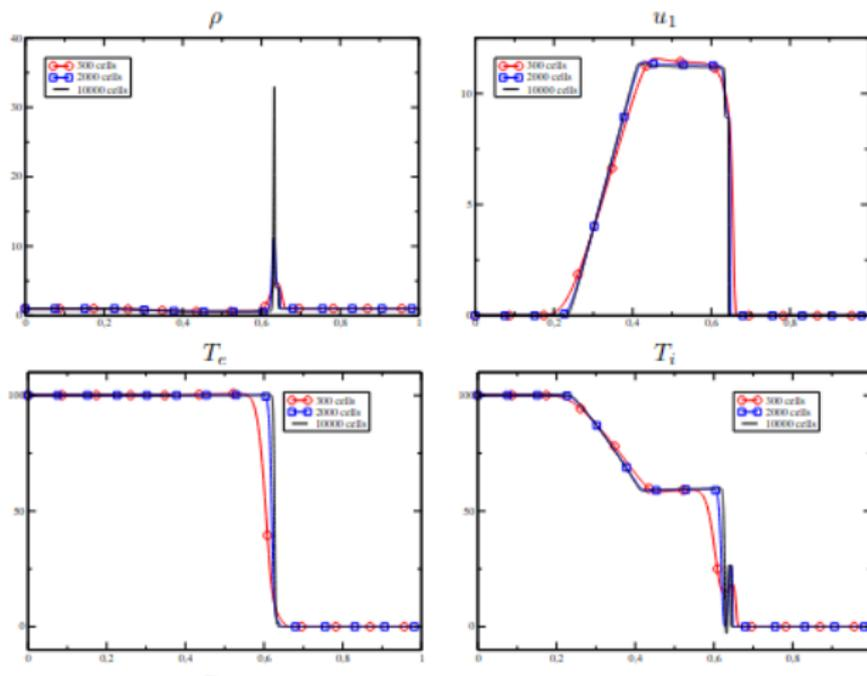
a right strong wave of shock, a right contact surface and a left rarefaction wave
