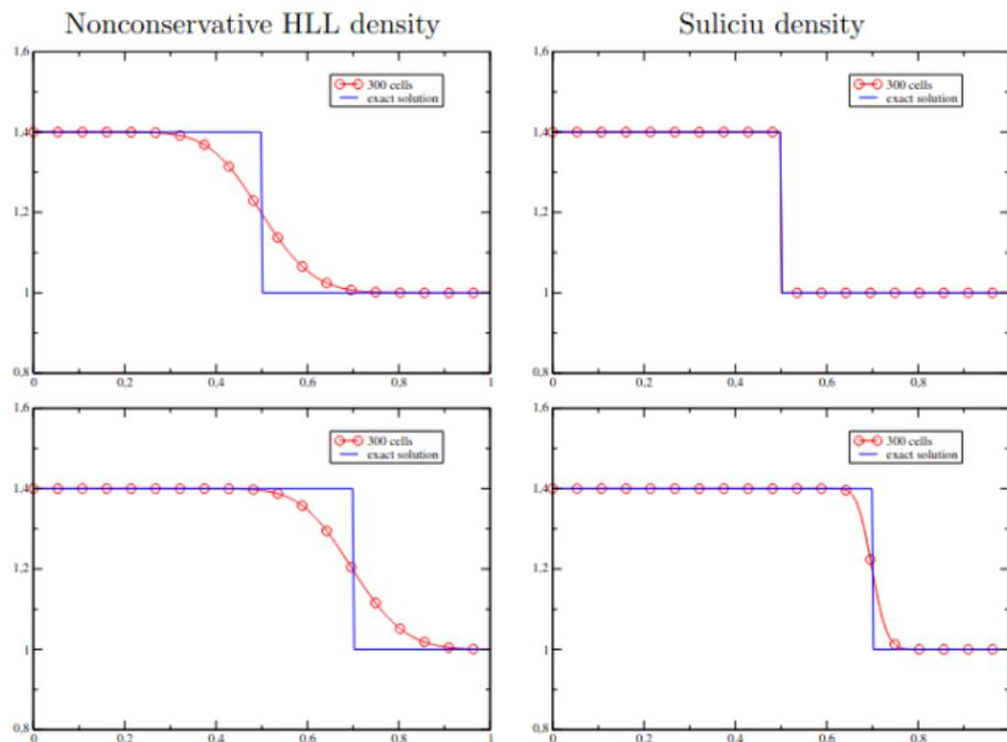
On the left, test 6 is an isolated stationary contact wave.
