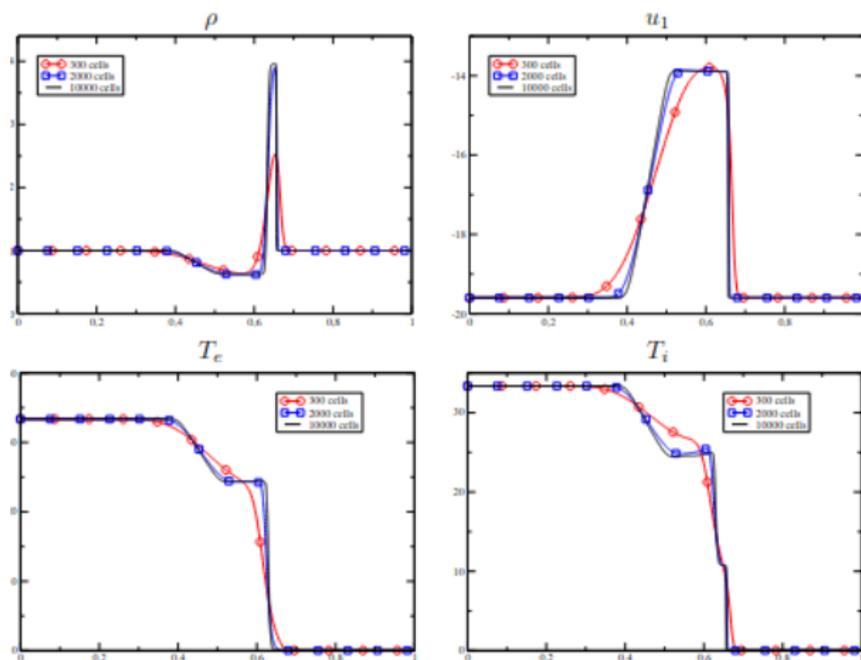
left rarefaction wave, a right-travelling shock wave and a stationary contact discontinuity
