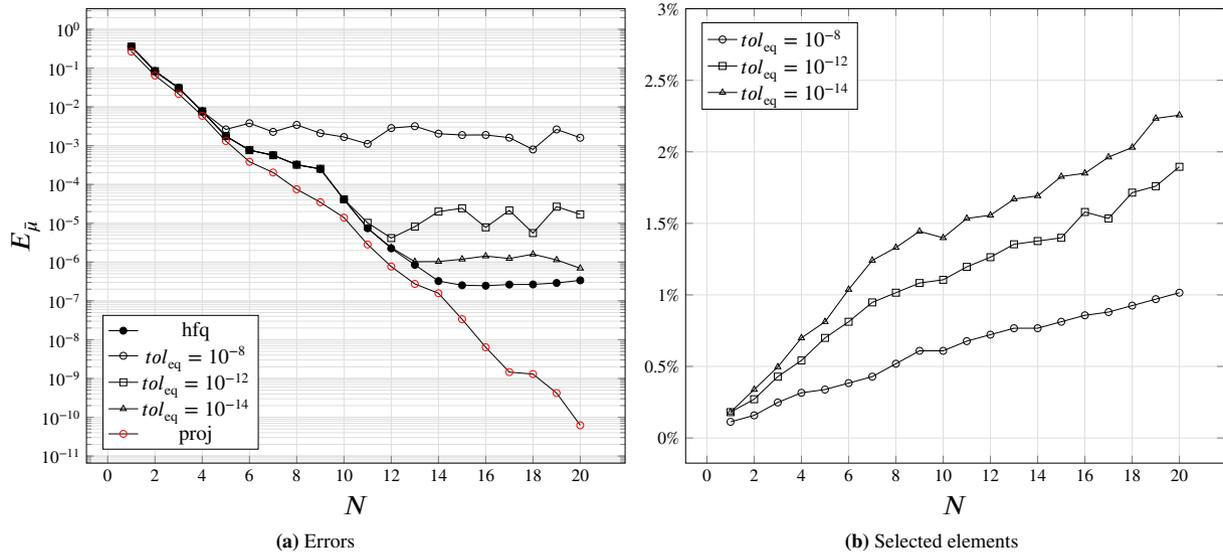
**FIGURE 3** solution reproduction problem. (a): errors associated to projection error (proj), Galerkin with high-fidelity quadrature (HFQ) and Galerkin with empirical quadrature for several choices of  $tol_{eq}$  with respect to the ROM dimension  $N$ . (b): percentage of selected elements for several  $tol_{eq}$ .
