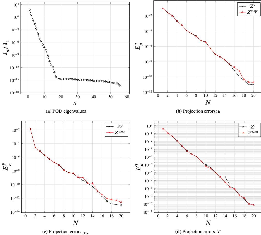
**FIGURE 2** solution reproduction problem. (a): exponential decay of POD eigenvalues. (b), (c), (d): projection errors computed through (35) (in black) and (36)-(38) (in red) for increasing numbers of POD modes.
