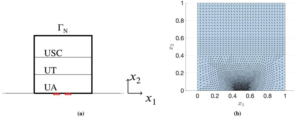
**FIGURE 1** geometric configuration: (a) the non-dimensional domain (b) the mesh. The size of each alveolus is equal to  $l_Q = 3.09$  [m], while the distance between consecutive alveoli is equal to  $l = 6.18$  [m].
