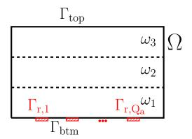
Figure 2: global system.  $\Gamma_{\text{top}}$  and  $\Gamma_{r,1}, \ldots, \Gamma_{r,Q_a}$  are associated with the stress conditions; the regions  $\{\Gamma_{r,q}\}_q$  are of equal size  $\ell_r > 0$ , and the distance between consecutive regions is constant and equal to  $\ell_r > \ell_r$ .
