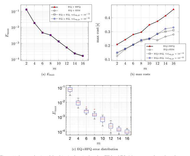
Figure 11: hyper-reduction of the objective function based on EIM and EQ. (a) worst out-of-sample performance of the hyper-reduced OS2 ROM for several choices of m, with n=m. (b) maximum computational cost over the test set. (c) Out-of-sample error distributions for the EQ+HFQ case. Results are based on the EQ tolerance  $tol_{\rm eq}=10^{-10}$  for the local problems and the tolerances  $tol_{\rm eq,p}=10^{-4}$  and  $tol_{\rm eq,p}=10^{-6}$  for the objective function (for EQ+EQ).
