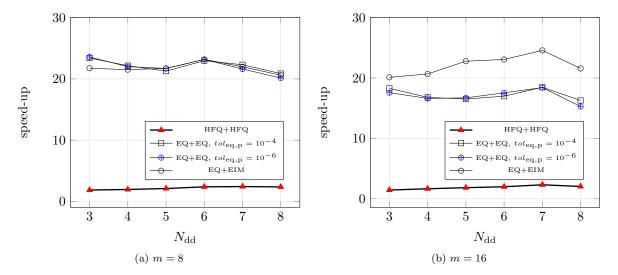
Figure 12: Speed-up of the OS2 ROMs with respect to the HF monolithic solver for several values of the number of subdomains. (a) performance for m = 8; (b) performance for m = 16. EQ tolerance for the port-to-bubble maps is set equal to  $tol_{eq} = 10^{-10}$ .
