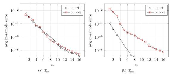
Figure 5: behavior of the average squared in-sample error  $E_n = 1 - \frac{\sum_{i=1}^{n} \lambda_i}{\sum_{j=1}^{n_{\text{train}}} \lambda_j}$  for several values of n, for port and bubble components, and for the two archetype components.
