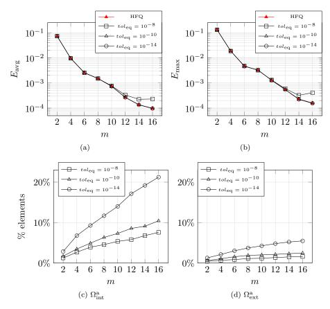
Figure 8: hyper-reduction of the port-to-bubble maps for several tolerances  $tol_{\rm eq}$  and port space sizes m, with n=m. Behavior of the (a) average, (b) max out-of-sample prediction. (c)-(d) percentage of sampled elements in  $\Omega_{\rm int}^{\rm a}$  and  $\Omega_{\rm ext}^{\rm a}$ .
