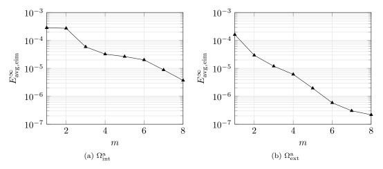
Figure 9: application of the EIM procedure for vector-valued fields (cf. Algorithm 3). (a)-(b) behavior of the in-sample  $L^{\infty}$  approximation error  $E^{\infty}_{\text{avg,eim}}$  for the internal and the external component.
