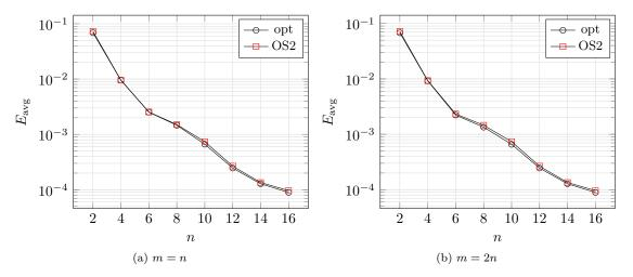
Figure 6: out-of-sample performance of OS2 ROM without hyper-reduction for several values of m, with n = m and n = 2m; comparison with optimal ("opt") average error  $E_{\text{avg}}^{\text{opt}}$  (42)
