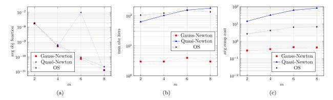
Figure 14: comparison between Gauss-Newton, quasi-Newton methods, and multiplicative overlapping Schwarz methods with zero initial condition. (a) average value of the objective function with respect to m and for n=m. (b) maximum number of iterations to meet the convergence criterion. (c) average wall-clock cost with respect to m and for n=m.
