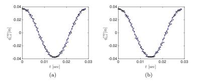
Fig. 2: Microtruss experiment. Time-harmonic  $x_2$ -displacement of blocks (1, 4) and (4, 4) in absence of added masses. The shaker input is displacement:  $A^{\text{dim}} \cos(2\pi f t) \mathbf{e}_2$ ,  $A^{\text{dim}} = 0.02$ [in], f = 35 [Hz].
