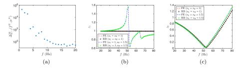
Fig. 6: Microtruss experiment: RB Approximation. Figure (a): convergence of the weak-Greedy. Figures (b) and (c): comparison between FE and RB feature predictions for  $\alpha = 5 \cdot 10^{-4}$ ,  $\beta = 10^{-4}$ ,  $E = 2.8 \cdot 10^9$  and three different choices of the geometric parameters.
