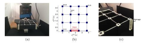
Fig. 1: Microtruss experiment. Figure (a): experimental apparatus. Figure (b): schematic of undamaged configuration at rest. Figure (c): detail of the added mass on top of block (1, 4).
